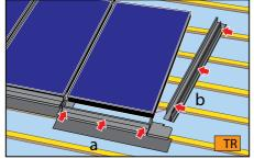
Push the sill flashing (2) into the gasket at the bottom of the solar panel. Push the lower side flashing (3) into the gasket on the right hand side of the panel.
