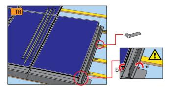
Fit the lower gutter (7), (16) and lower gutter covers (8). See steps 10 and 11.
