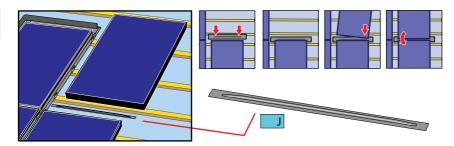
Push the joining strip (6) into the gasket in the top edge of the panel below and slide the solar panel in to engage with the joining strip and combi-brackets on two sides.
