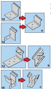
Where the roof has sarking boards, special kits are available for fixing. Fixing brackets replace those in the standard kit as shown. Align the brackets (a, b) top and bottom to fix through into rafters.
