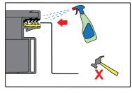
Fit the sill flashing (2) then the lower side flashing (3) to the panel. Flashings push into the rubber gasket seal in the upper slot of the panel frame. Take care to align the leading edge just above the yellow line on the gasket. Use soapy water or glass cleaning fluid to lubricate.
