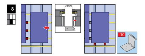
Slide the first panel of the next column sideways to engage with the combi-batten brackets. The bracket sets the gap to 30 mm. Secure the new solar panel to each rafter it crosses with rafter brackets (12) and two 50mm screws (20) each.
