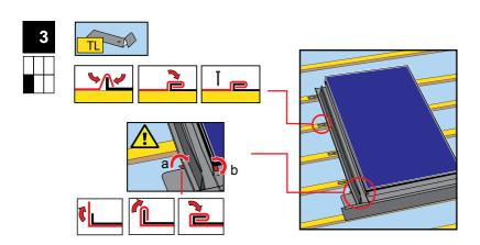
Secure the edge of the side flashing using side fixing tabs (17) and nail (18). Fold over the tab on the sill flashing (a) to grip the side flashing. Fold down the tab on the side flashing (b).
