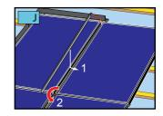
Fit gutter cover (10) into the panel gasket. Fold the end of the joining strip down into the gutter.
