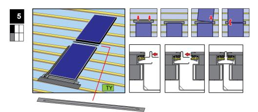
Push the joining strip (6) into the gasket on the top face of the lower solar panel. Align to the centre of the panel.
