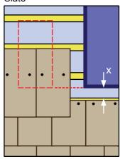
For best results align the bottom edge of panel with the slate line. This may require that slates below the panels are nailed in advance. If installing before slating, set x to 130mm.
