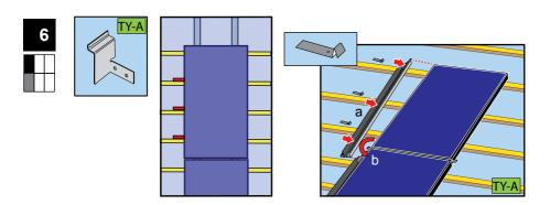
Fix the left side of the solar panel with batten brackets (14) and 25mm screws (19). Push in the upper side flashing (4) and fix the outside edge with side fixing tabs (17).
