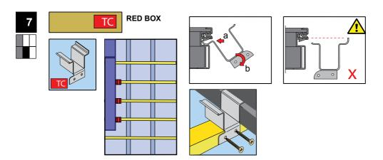
Fix combi-batten brackets (15) to the right hand side of the bottom solar panel. The bracket must be turned so that the side with the taller edge goes into the panel. Fix each brackets with two 25mm screws (19).
